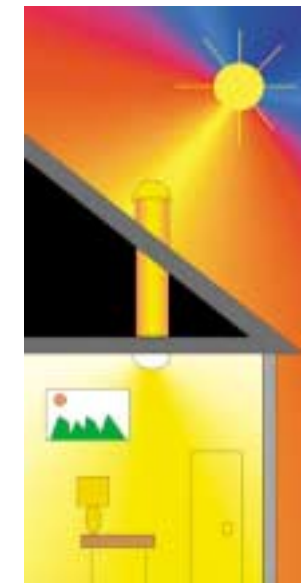
A tubular skylight funnels daylight to a ceiling diffuser.
